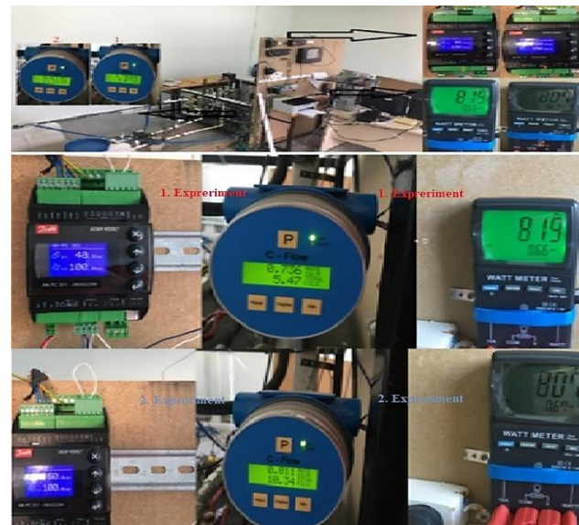
Figure 3. Pressure, mass CO2 flow and total power consumption in the test system (ISUBÜ CO2 Laboratory)
