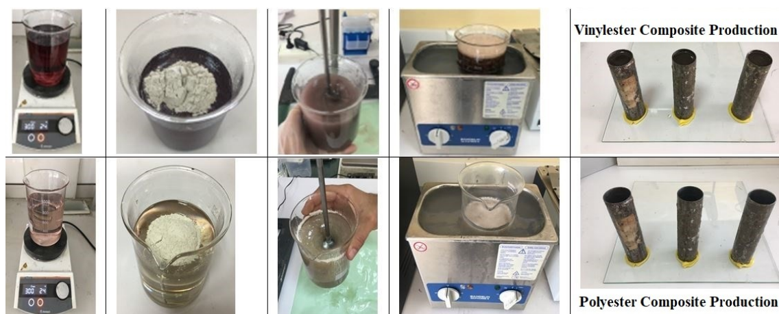
Figure 1: Preparation of tincal-reinforced vinylester and polyester composites.
