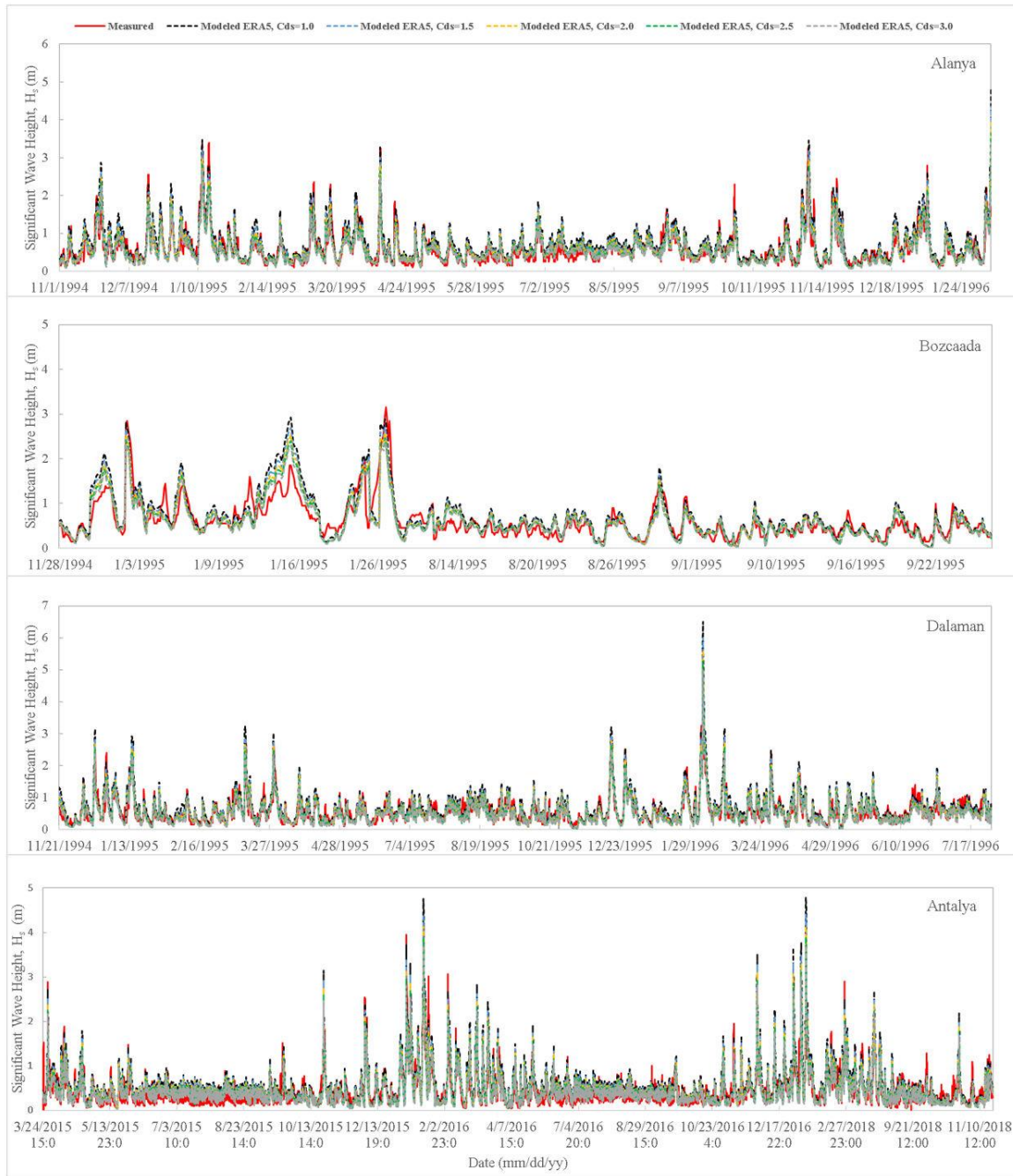
Fig. A.1. Comparison between significant wave heights modeled using ERA5 wind fields and measured at Alanya, Bozcaada, Dalaman, and Antalya stations.
