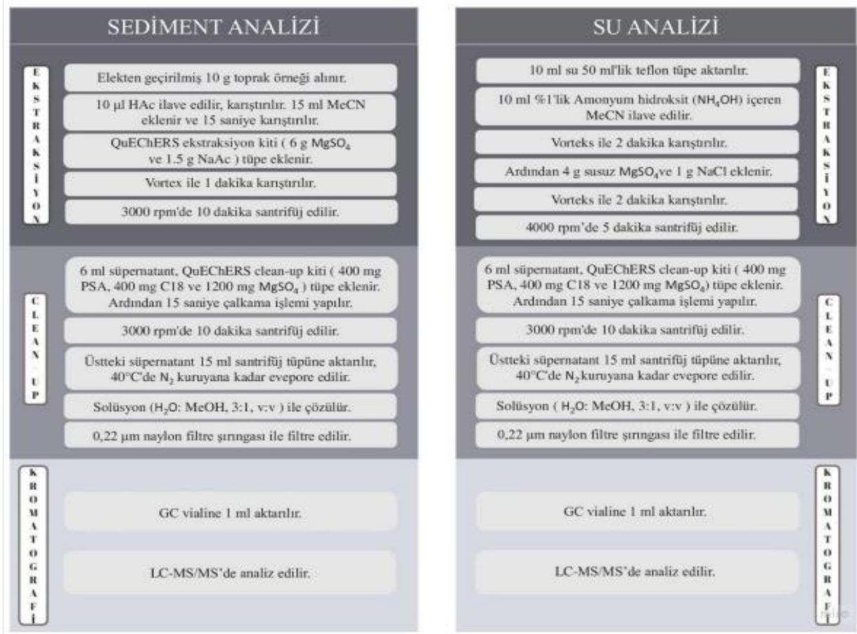
Figure 1. Analytical steps of the QuEChERS method followed in the analyzes.
