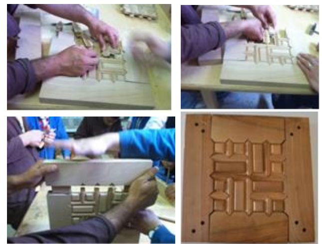
Figure 8. The general assembling procedure of the original "Kündekari" panel
