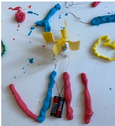
Photograph 5a. Conductive play dough DC motor circuits
