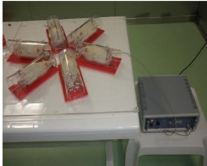
Fig 3. Plastic Tube and Monopole Antenna Assembly in which the Rats are Placed
