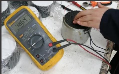
Figure 6. Measuring voltage of the embedded piezoelectric sensors
