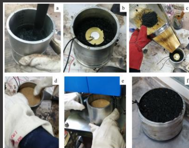
Figure 2. First experimental setup; a) Placing the asphalt mixture into the mold, b) Placing the piezo on the mixture, c) Covering the mixture on which the piezo is placed with mastic, d) placing the cork on the sample before compaction, e) Compaction the sample, f) Sample after compaction.
