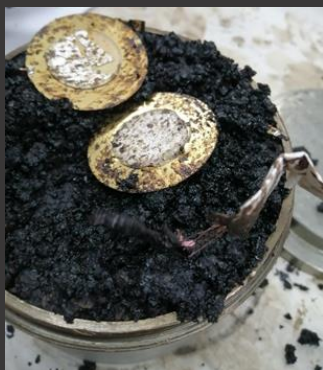
Figure 7. Damaged series-connected piezo electric sensor after the Marshall compaction phase
