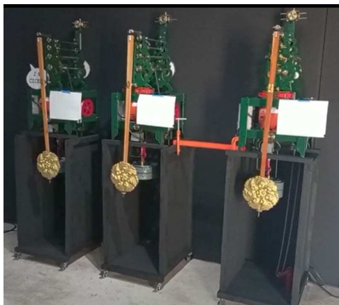
Figure 2 Modern version of the Huygens experiment, synchronizing two monumental clocks. Note that the means of communication between the two clocks is the orange wooden stick.
