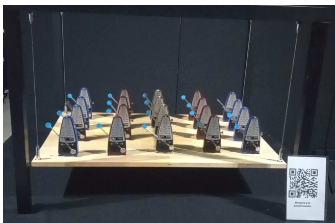
Figure 3 Hanging platform with synchronized metronomes (Echenausía-Monroy 2022c).
