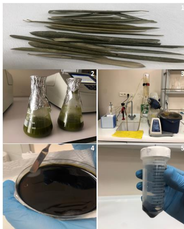
Figure 1. Process of Olive leaf methanol extract preparation; 1: Olive leaves, 2: Homogeneous extract, 3: Evaporator device, 4: Planning by scraping the dried extract, 5: Extract transferred to test tube.
