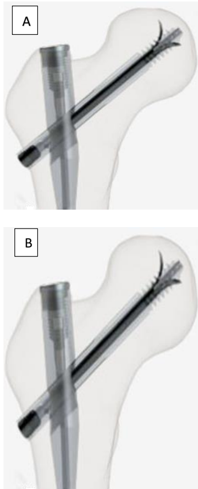
Figure 2. Lag screw differences of proximal femoral nails used in bone models A: lag screw with blade B: anti-rotatory lag screw
