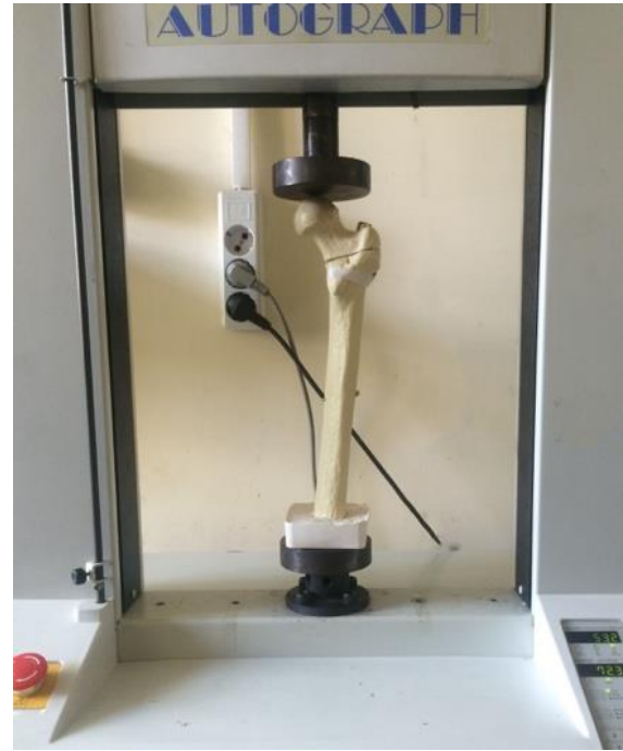
Figure 3. Bone model during axial loading
