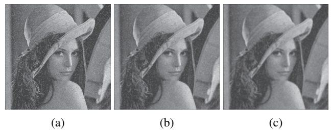
Figure 9. The noise reduced images obtained by using filter operators with sized (a) 3 \times 3 (b) 5 \times 5 (c) 7 \times 7 from noise density 0.05 image.
