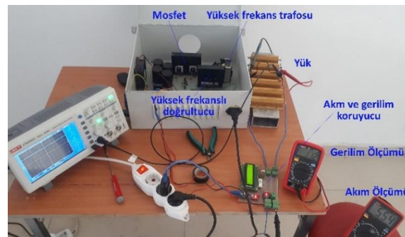
Figure 19. Application setup and measurements.
