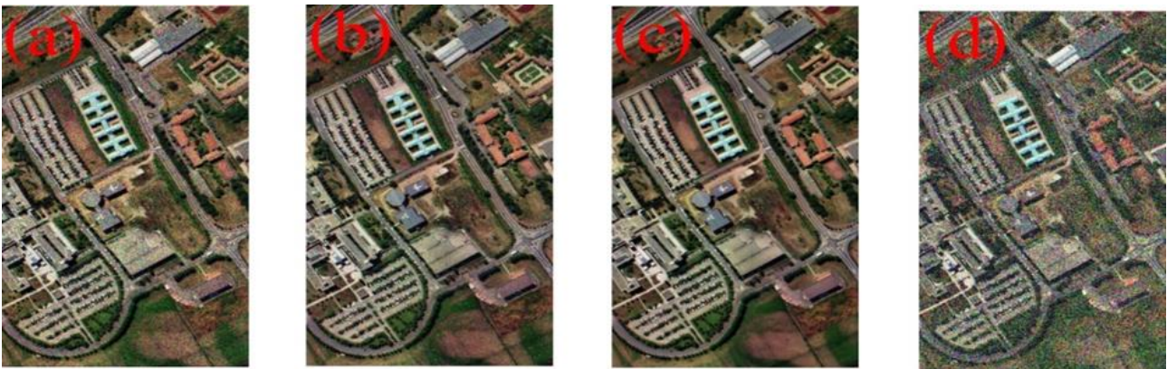
Figure 3. RGB image of HSI with noise added a) Speckle, b) Salt & Pepper, c) Poisson and d) Gaussian
