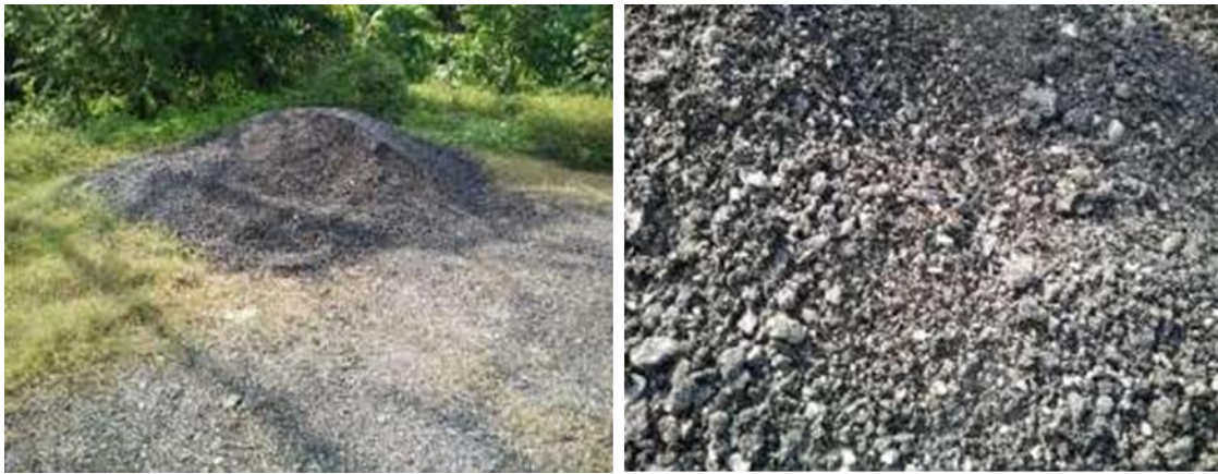
Figure 2.2: Abandon Reclaimed Asphalt Pavement (RAP)
