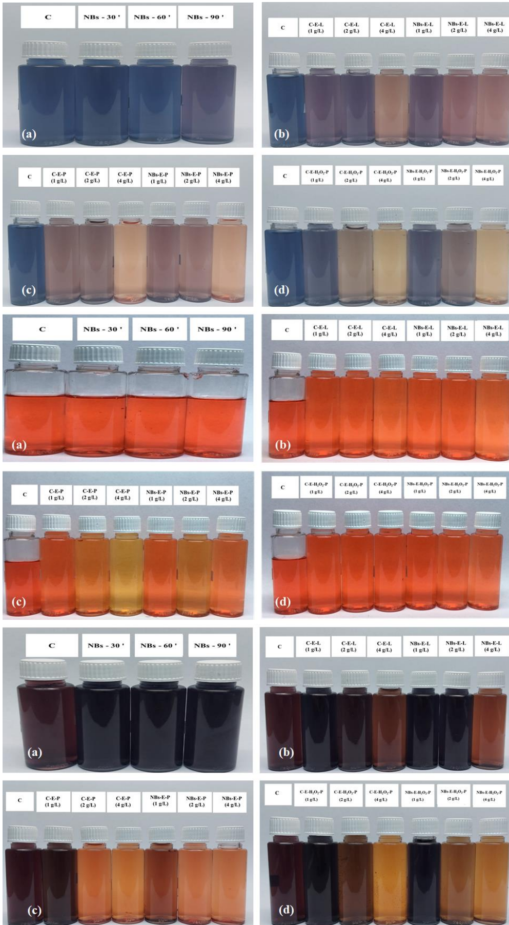
Figure 8. Images of the decolorization processes of dark shade blue (top), red (middle), and black (bottom) dyeings: (a) NBS, (b) C/NBS-E-L, (c) C/NBS-E-P, (d) C/NBS-H 2 O 2 -E-P
