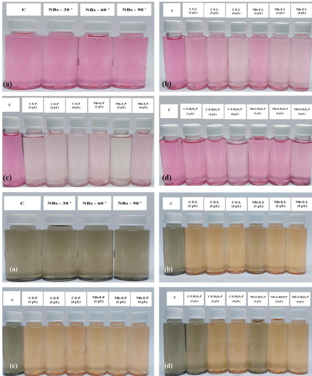
Figure 4. Images of the decolorization processes of light shade fuchsia (top) and navy blue (bottom) dyeings: (a) NBs, (b) C/NBs-E-L, (c) C/NBs-E-P, (d) C/NBs-H 2 O 2 -E-P
