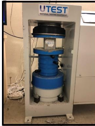
Fig. 4 Compressive strength test device
