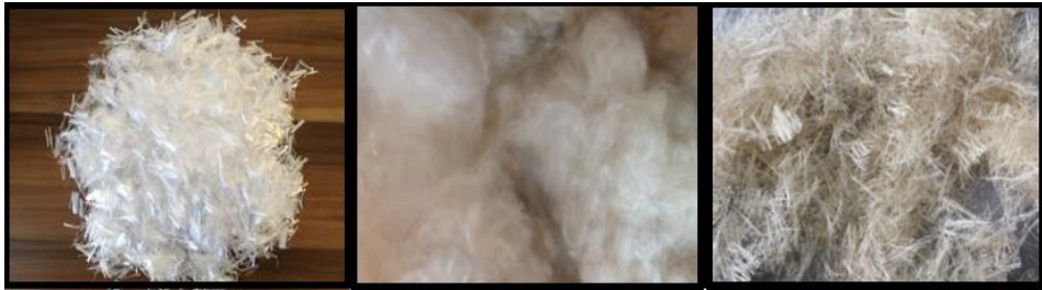
Fig. 1 Polypropylene Fiber, Kapok Fiber and Coconut Fiber
