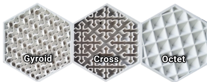
Figure 1 Unit cell structures used for infills [13].
