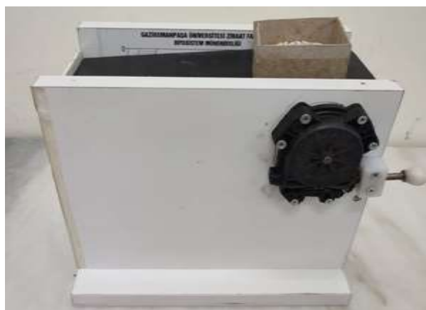
Figure 2. Measuring device for the coefficient of the friction
