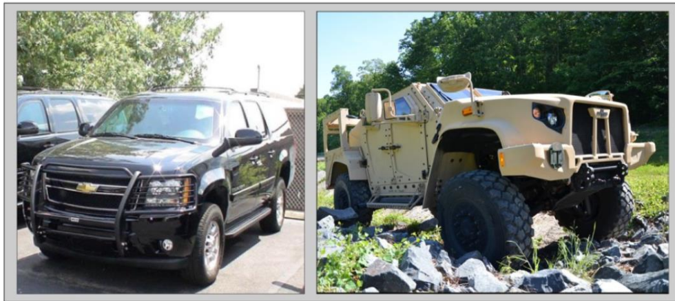
Figure 10: Typical Armored Commercial Passenger-Carrying Vehicle (left) Compared with Tactical Vehicle (right) (Source: United States Government Accountability Office, 2017)
