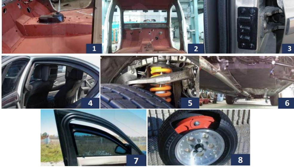
Figure 19: Armoring of a Civilian Vehicle
