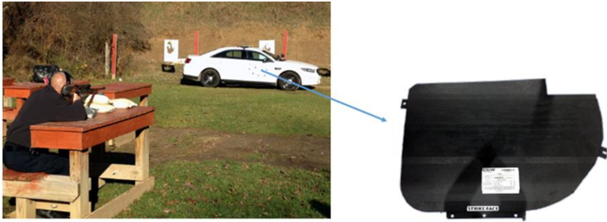
Figure 16: Ballistic Door Panel Produced by Dew Engineering and Development Company (Source: DEW Engineering and Development, n.d.a)
