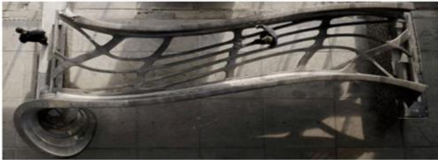
Şekil 23. WAAM katmanlı imalat sisteminde üretilen metal köprü (Çelik vd., 2017) Figure 23. Metal bridge fabricated on the WAAM additive manufacturing system (Çelik et al., 2017)
