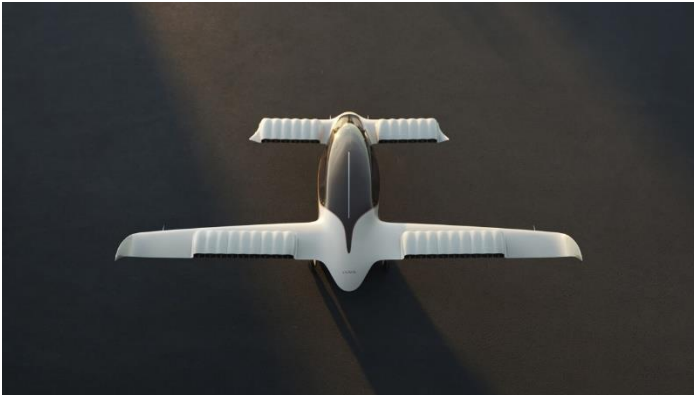
Şekil 10: Lilium Açılı İtme/Çekme (Vectored Thrust) eVTOL ( https://lilium.com/jet , 06/09/2022).
