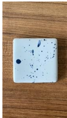
Figure 5. Faults due to splash of colored glaze.
