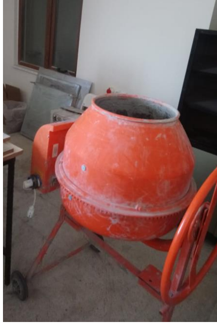
Figure 1. Laboratory type concrete mixing machine
