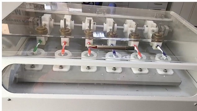
Figure 3. Toothbrushing simulation device used in the study
