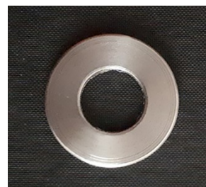
Figure 1. Stainless-steel mold for conventional PMMA and bis-acryl composite resin materials
