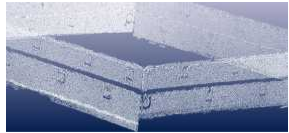
Figure 8. Point Cloud produced by MVS from SURF results.
