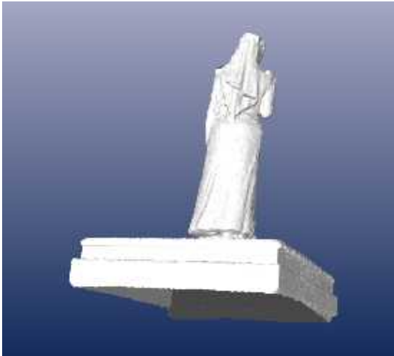
Figure 10. 3D model obtained from %20 compressed images by SURF.
