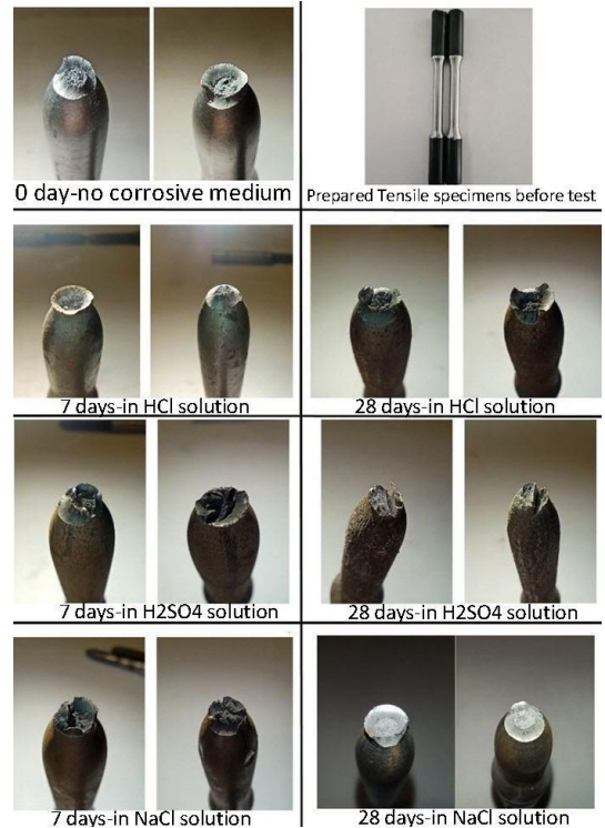
Figure 11. Fractured surface of tensile specimens
