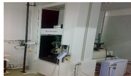
Figure 4. Test setup for the axial compression
