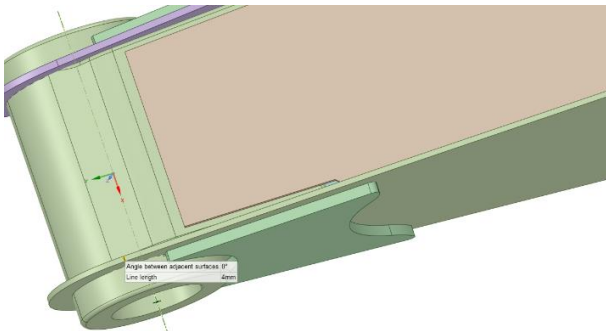
Fig. 4. Side plate thinned from 5 mm to 4 mm
