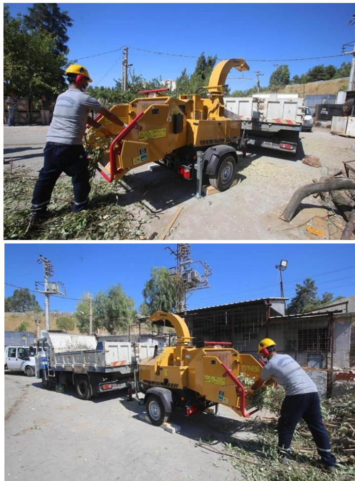
Figure 2. Studies on the grinding of wood cutting residues with a gasoline-powered grinder (Karabaglar, 2021).
