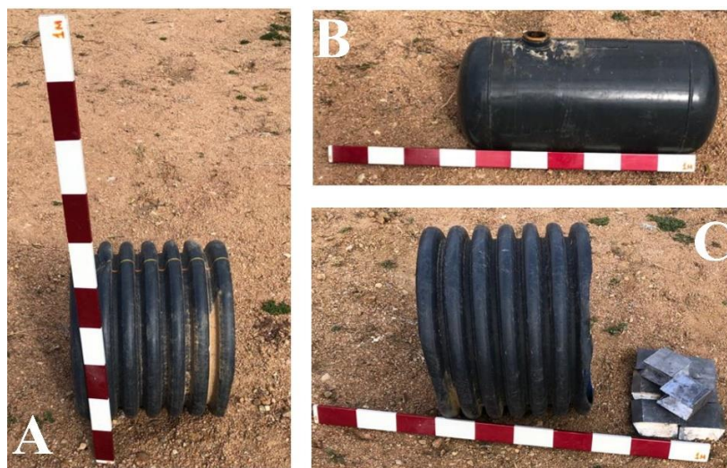
Figure 3. Objects with different material properties to be buried in the test site
