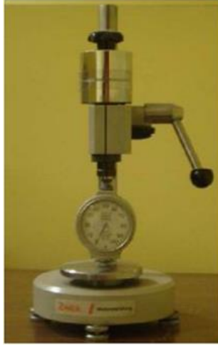
Fig. 8. Shore-D Test Device.
