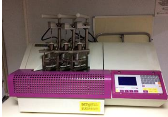
Fig. 10. Heat Deformation (HDT) Testing Machine.
