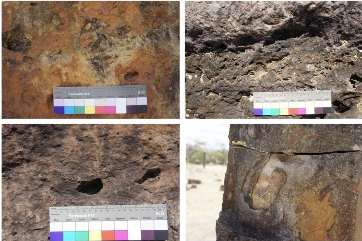
Figure 9. Relief caused by out-weathering of fossil components (upper left) and alveolar weathering (upper right); cavernous weathering (down left) and bursting on the monoliths
