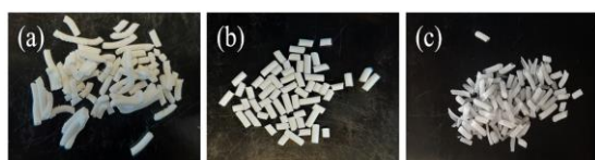
Figure 8. Images of the extrudates peptized with (a) 0 \text{HNO}_3/\text{AlOOH} , (b) 0.017 \text{HNO}_3/\text{AlOOH} , (c) 0.054 \text{HNO}_3/\text{AlOOH} molar ratios
