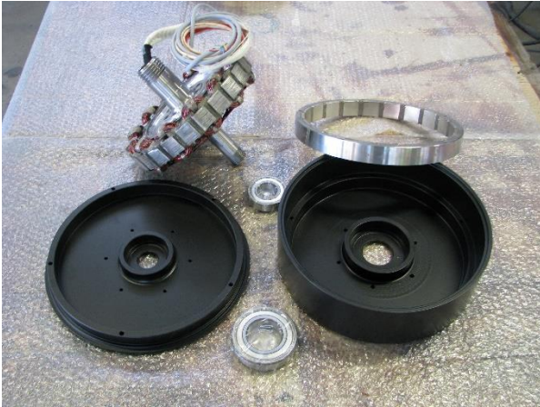
Figure 7. Stator with completed wound
