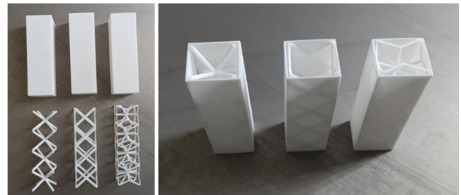
Fig. 5. Tubes, lattice and hybrid structures produced by additive manufacturing method
