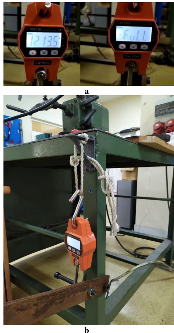
Figure 10. The load that the 90-90 mm bracket (a) fails at, and the 155-135 mm bracket withstands (right), the test setup for the experiment (b).
