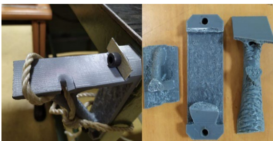
Figure 7. Failure resulting from incorrect placement of the load.
