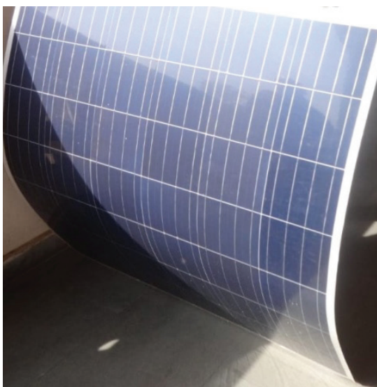
Figure 2. Flexible structure of PV module.
