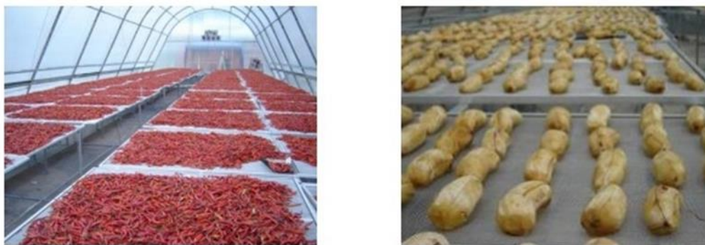
Figure 13. Interior view of a greenhouse dryer for drying chilli (a) and banana (b) ( Intawee et al., 2011 ).
