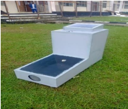
Figure 2. Indirect active solar dryers ( Alonge and Jackson, 2014 ).
