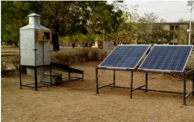
Figure 6. A hybrid photovoltaic (PV) solar dryer ( Hussien et al. , 2017 ).
