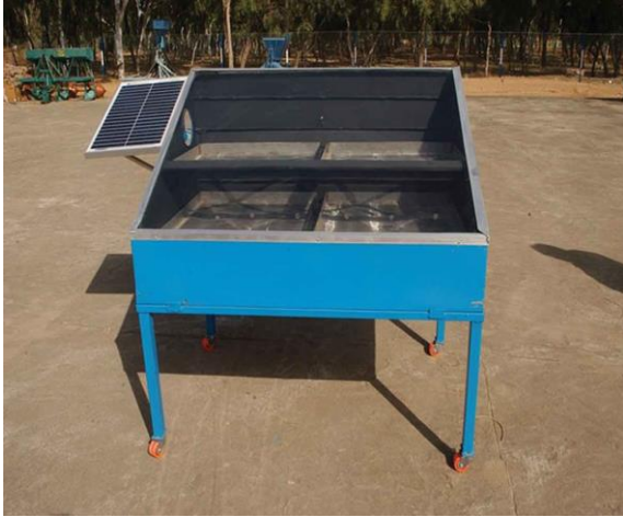
Figure 4. PV/T hybrid solar dryer ( Poonia et al., 2018 ).
