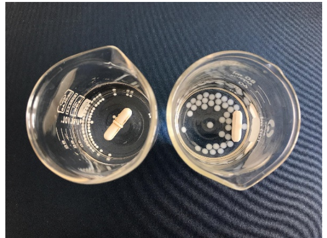
Fig.3. Swelling was observed when the vitamin C microcapsules were kept at pH: 7.35 in an aquatic environment for 8 hours (in the right beaker).
