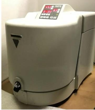
**Figure 1.** Shows planetary mono mill pulverisette 6 classic line
