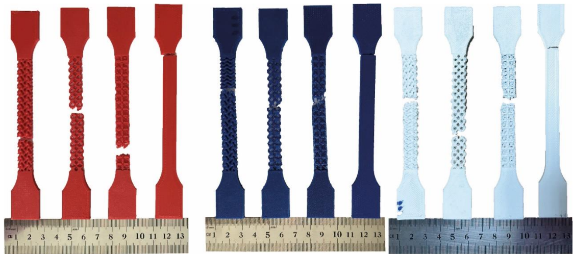
Figure 7. Deformation images after tensile test
