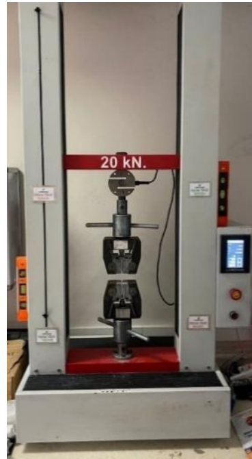
Figure 2. Tensile test device used for testing specimens (Labomak)
