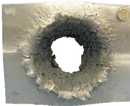
Figure 1. Deformation on a 50 mm Thick Aluminum Plate Due to an Impact by a 10 g Lexan Slug at 7 km/s (Christiansen and Calhoun 2017)
