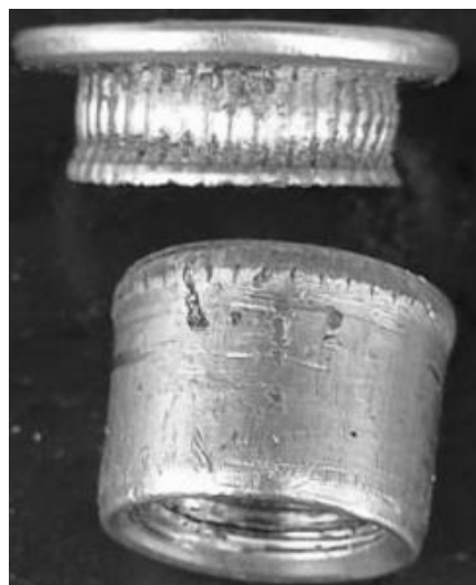
Figure 8. Failure mode in the BRN of S10 ( t_w=5.00 mm and BRN-M12)
