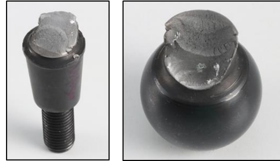
Fig. 15. Broken images of nitration treated joint
