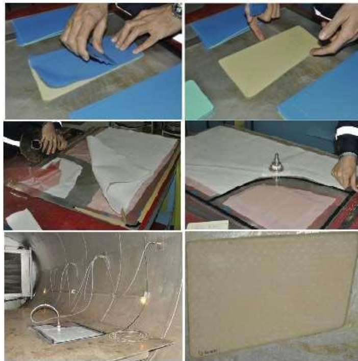
Figure 3. Composite Test Panel Manufacturing
