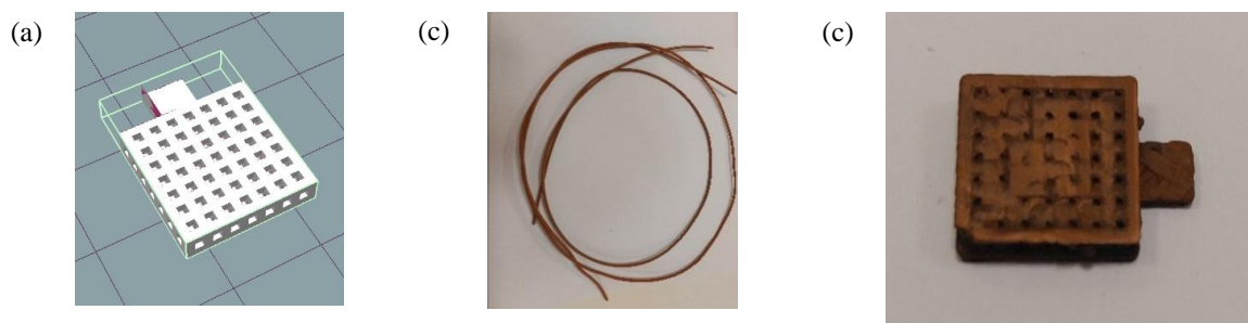
Figure 1. Electrode geometry designed with open-source FreeCAD (a), and images of Cu-PLA composite filament (b) and 3D Cu-PLA electrode (c).
