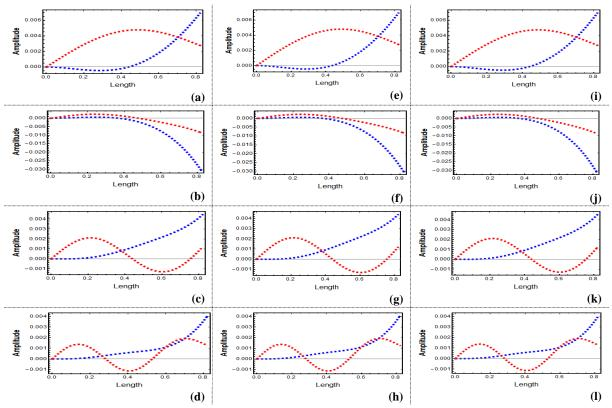
Figure 21. First four consecutive vibration mode shapes of an aircraft structure with semi-circle crosssection for S-S boundary condition (blue: bending, red: torsion), (a)-(d) when P = 0 N, (e)-(h) when P = 1790 N, and (i)-(l) when P = -1790 N
