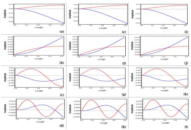
*Figure 19.* First four consecutive vibration mode shapes of an aircraft structure with semi-circle crosssection for C-F boundary condition (blue: bending, red: torsion), (a)-(d) when P = 0 N, (e)-(h) when P = 1790 N, and (i)-(l) when P = -1790 N
