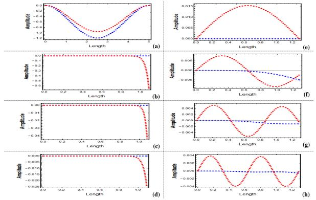
*Figure 17.* First four consecutive vibration mode shapes of an aircraft structure with channel crosssection for C-C boundary condition (blue: bending, red: torsion), (a)-(d) when P = 5.7645e + 04 N (i.e., the ultimate axial compression load), (e)-(h) when P = -7.6148e + 04 N (i.e., the ultimate axial tensile load)
