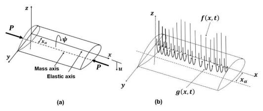
*Figure 2.* (*a*) a uniform axially loaded coupled bending-torsion beam on the coordinate system, (*b*) the distributed external forces and torques applied to the beam
