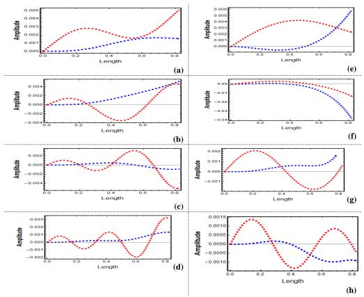
*Figure 24.* First four consecutive vibration mode shapes of an aircraft structure with semi-circle crosssection for S-S boundary condition (blue: bending, red: torsion), (a)-(d) when P = 6.6528e + 04 N (i.e., the ultimate axial compression load), (e)-(h) when P = -8.7883e + 04 N (i.e., the ultimate axial tensile load)
