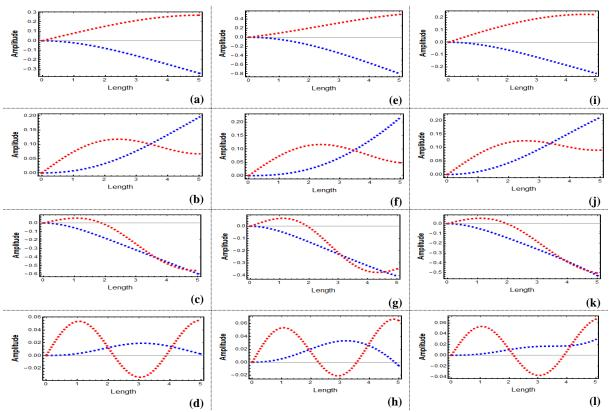
*Figure 25.* First four consecutive vibration mode shapes of an aircraft structure with open box crosssection for C-F boundary condition (blue: bending, red: torsion), (a)-(d) when P = 0 N, (e)-(h) when P = 2500 N, and (i)-(l) when P = -2500 N
