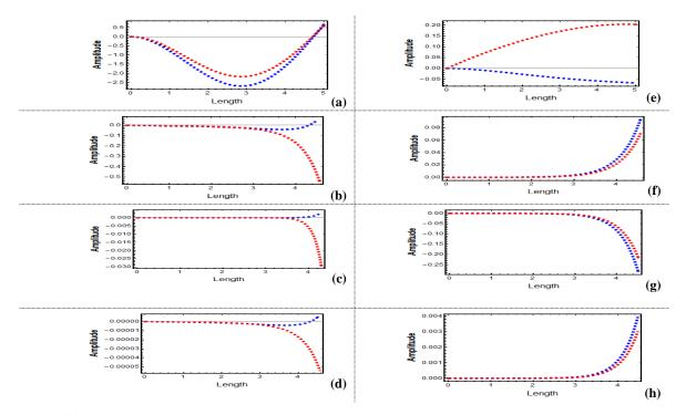
Figure 28. First four consecutive vibration mode shapes of an aircraft structure with open box crosssection for C-F boundary condition (blue: bending, red: torsion), (a)-(d) when P = 18.9216e + 04 N (i.e., the ultimate axial compression load), (e)-(h) when P = -24.9952e + 04 N (i.e., the ultimate axial tensile load)
