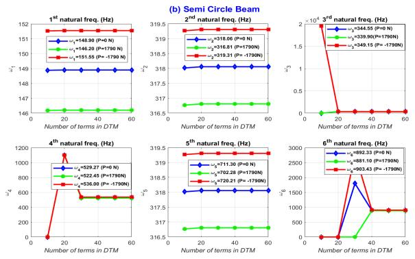
*Figure 11.* Convergence test for the aircraft structure with semi-circle cross-section for S - S boundary condition
