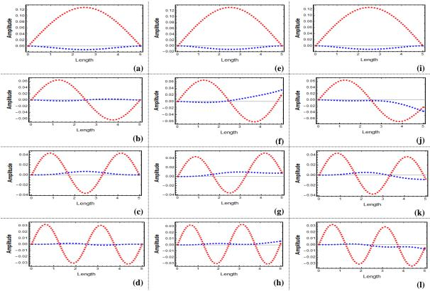
*Figure 26.* First four consecutive vibration mode shapes of an aircraft structure with open box crosssection for C-C boundary condition (blue: bending, red: torsion), (a)-(d) when P = 0 N, (e)-(h) when P = 2500 N, and (i)-(l) when P = -2500 N
