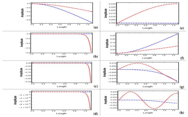
*Figure 16.* First four consecutive vibration mode shapes of an aircraft structure with channel crosssection for C-F boundary condition (blue: bending, red: torsion), (a)-(d) when P = 5.7645e + 04 N (i.e., the ultimate axial compression load), (e)-(h) when P = -7.6148e + 04 N (i.e., the ultimate axial tensile load)
