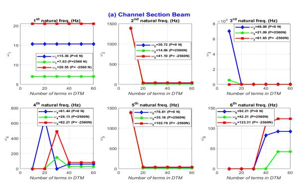
(ii) Convergence test for clamped-clamped (C-C) boundary condition
