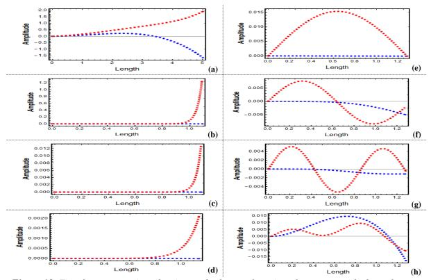
Figure 18. First four consecutive vibration mode shapes of an aircraft structure with channel crosssection for S-S boundary condition (blue: bending, red: torsion), (a)-(d) when P = 5.7645e + 04 N (i.e., the ultimate axial compression load), (e)-(h) when P = -7.6148e + 04 N (i.e., the ultimate axial tensile load)
