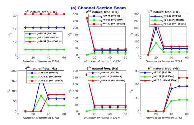
*Figure 10.* Convergence test for the aircraft structure with channel cross-section for S - S boundary condition
