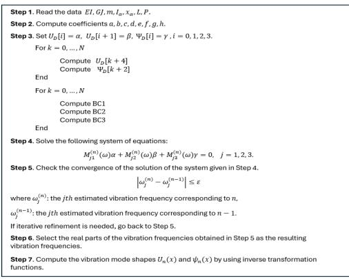
Algorithm 1. The pseudocode of DTM ( $\varepsilon$ : is a tolerance value, BC: boundary condition)
