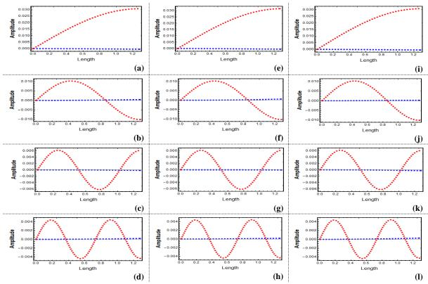
**Figure 13.** First four consecutive vibration mode shapes of an aircraft structure with channel crosssection for C-F boundary condition (blue: bending, red: torsion), (a)-(d) when P = 0 N, (e)-(h) when P = 2560 N, and (i)-(l) when P = -2560 N
