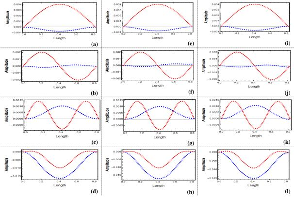
*Figure 20.* First four consecutive vibration mode shapes of an aircraft structure with semi-circle crosssection for C-C boundary condition (blue: bending, red: torsion), (a)-(d) when P = 0 N, (e)-(h) when P = 1790 N, and (i)-(l) when P = -1790 N
