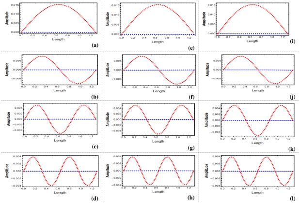
**Figure 15.** First four consecutive vibration mode shapes of an aircraft structure with channel crosssection for S-S boundary condition (blue: bending, red: torsion), (a)-(d) when P = 0 N, (e)-(h) when P = 2560 N, and (i)-(l) when P = -2560 N
