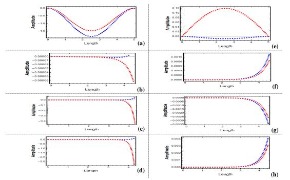
Figure 29. First four consecutive vibration mode shapes of an aircraft structure with open box crosssection for C-C boundary condition (blue: bending, red: torsion), (a)-(d) when P = 18.9216e + 04 N (i.e., the ultimate axial compression load), (e)-(h) when P = -24.9952e + 04 N (i.e., the ultimate axial tensile load)
