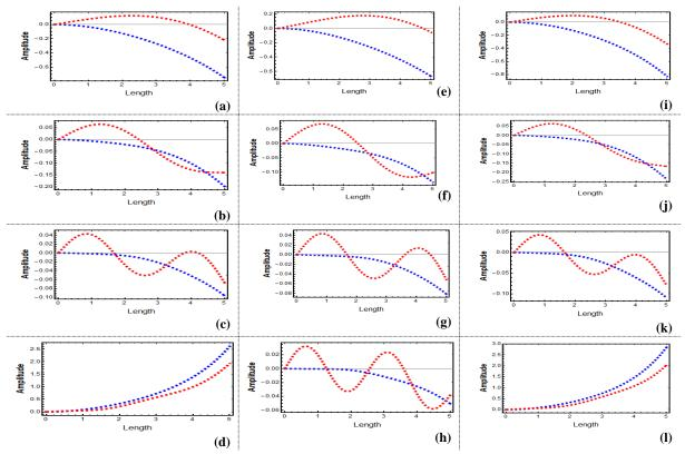
**Figure 27**. First four consecutive vibration mode shapes of an aircraft structure with open box crosssection for S-S boundary condition (blue: bending, red: torsion), (a)-(d) when P = 0 N, (e)-(h) when P = 2500 N, and (i)-(l) when P = -2500 N
