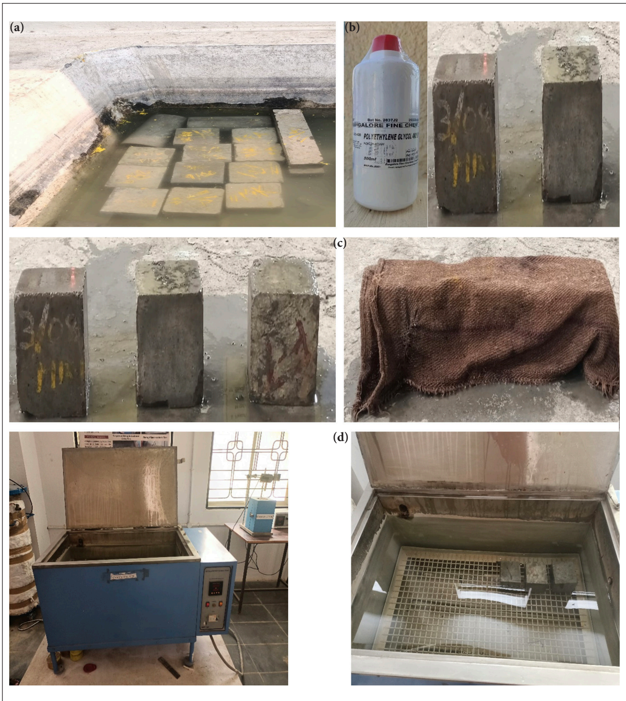
Figure 3. (a) Water immersion curing. (b) Self-curing with PEG-400. (c) Gunny bag membrane curing. (d) Accelerated curing.
