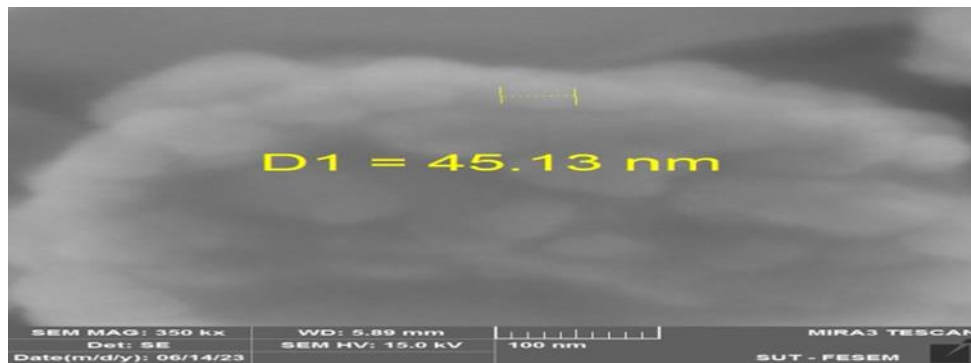
Figure 7: (SEM) of the nano-sulfur prepared from K2SX.
